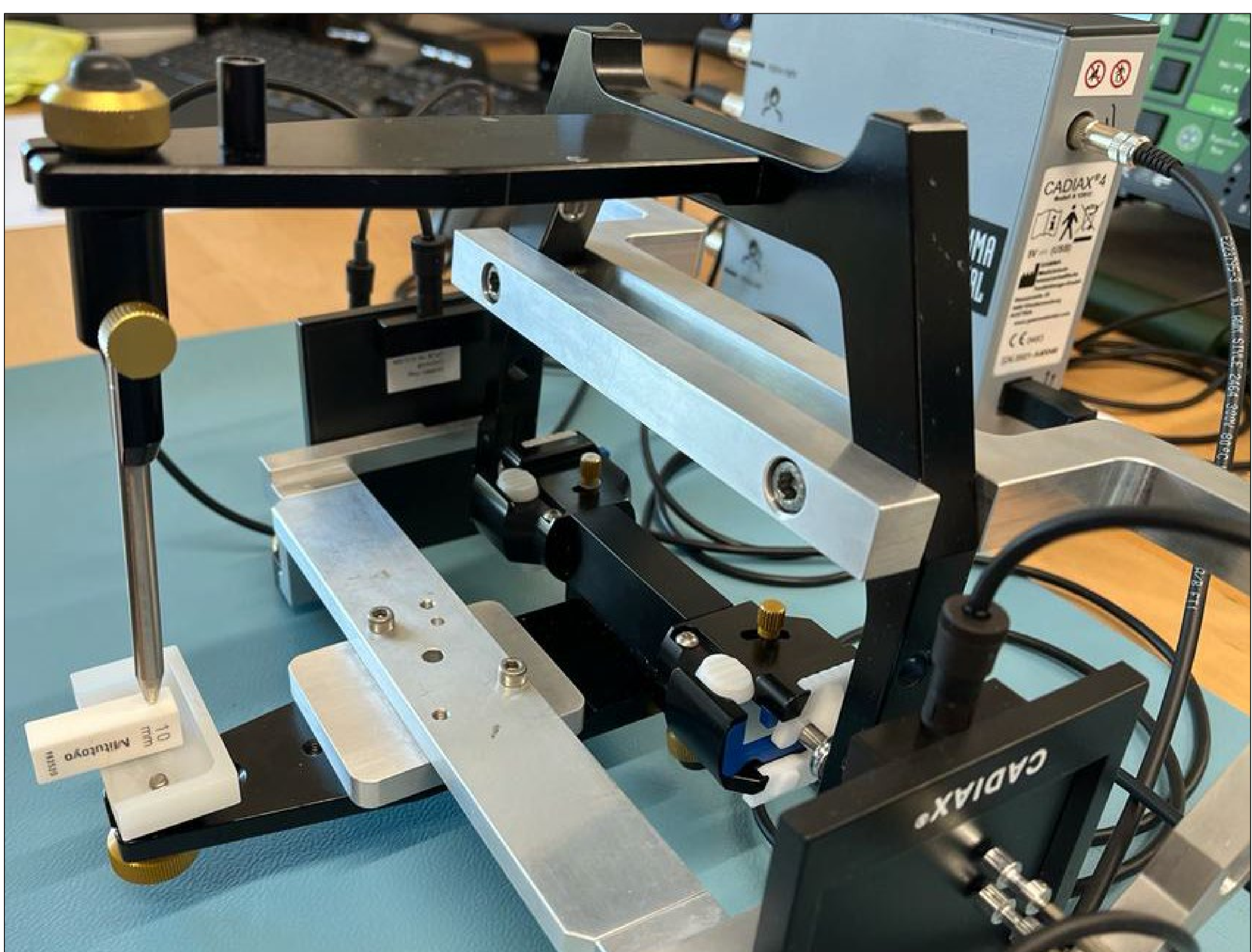
Figure 2: Measurement setup with the articulator positioned upside down and the parallel gauge block placed on the incisal table. The articulator was opened at predetermined distances from incisal pin using calibrated parallel gauge blocks of known heights.
